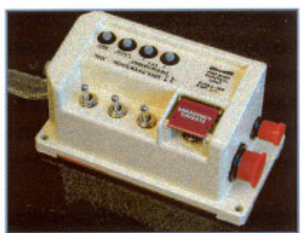
Engine bay control unit
